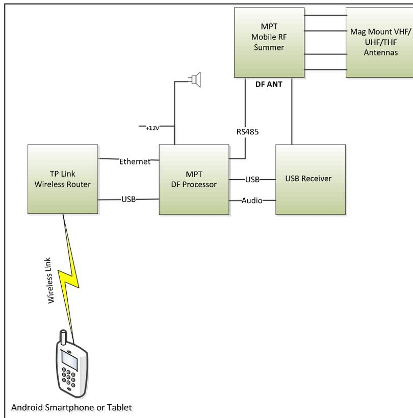
Figure 1: Block Diagram of Hardware Setup
