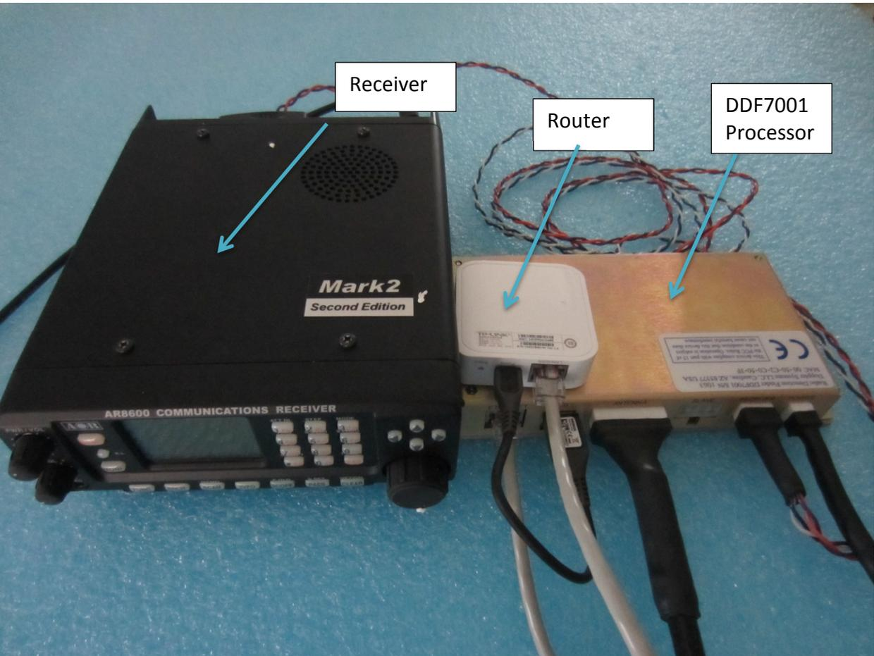
Figure 2: Typical Hardware Setup for Wireless Control
